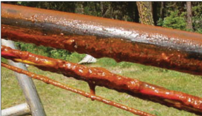
FIGURE 3 Biofilm on well wiring
